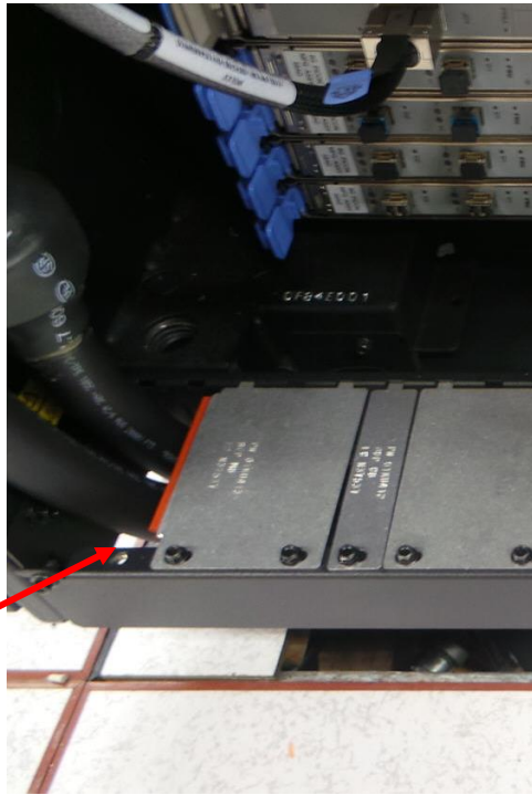
Figure 18: Line Cords in Strain Relief Clamp for Bottom Exiting System
